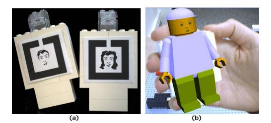
Figure 2. The dolls: (a) LEGOman and LEGOwoman with attached markers; (b) User carrying the augmented LEGOman.
